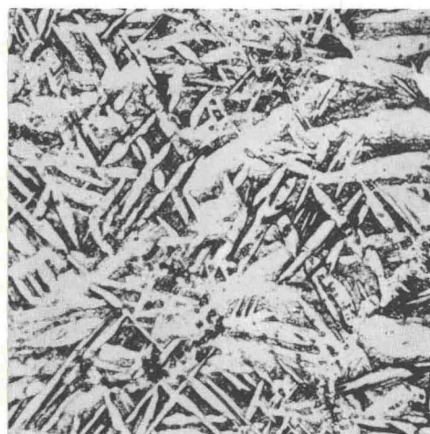
Fig. 12 Titanium-(2 wt per cent magnesium). Prepared by melting bulk components at 1900^{\circ}\text{C} , 100,000 atm and cooling under pressure. 500X
