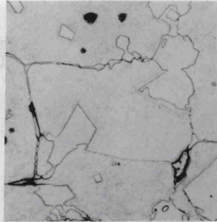
Fig. 18 High-speed tool steel. Heat treated at atmospheric pressure. Preheated at 1500°F. Austenitized at 2400°F and air cooled. 750X
